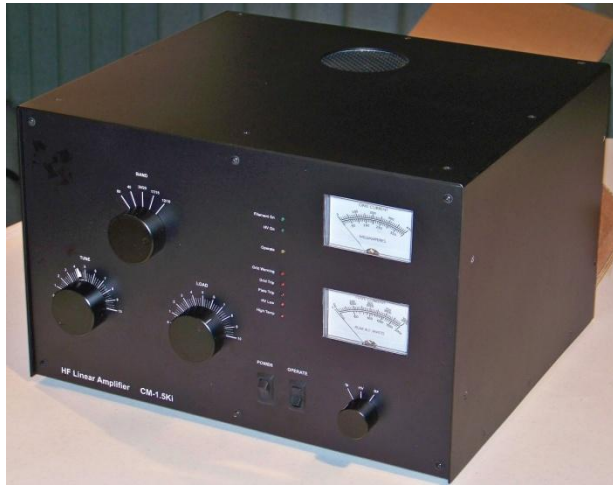
Mike's complete all-band HF linear amplifier.
