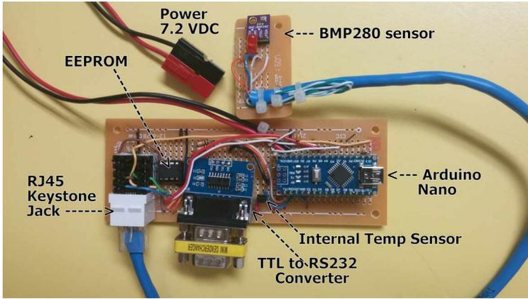
**Arduino-based Control Board**
