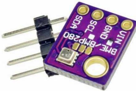
**Figure 3: Bosch BME280 Temp., Humidity, & Pressure Sensor**
