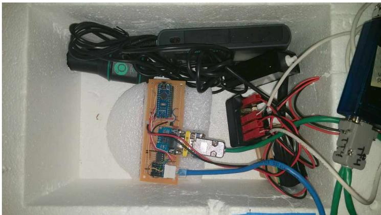
**RHS Instrument, Arduino & Li-Ion Batteries**
