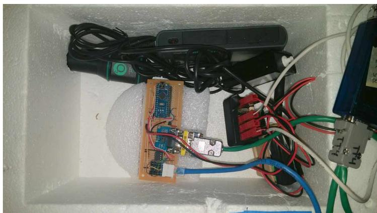
**RHS Instrument, Arduino & Li-Ion Batteries**
